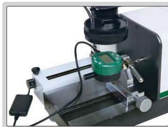
check INSIZE digital indicators (connection with cable)
