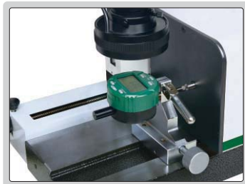
check digital indicators (detect digits on screen)
