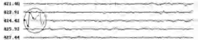
Picture 37 Special broken wire signals (Yuyang Coalmine hoisting rope)
